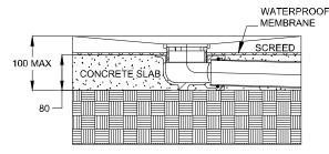
Connect the threaded body (not supplied) to the cast iron body and adjust the height to the required FFL.
